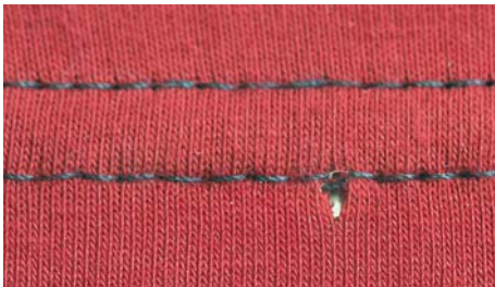
STITCHES IN THE KNITTING ARE DAMAGED – TEST IS CONTINUED WITH THE NEXT SIZE DOWN OF NEEDLE THICKNESS.
