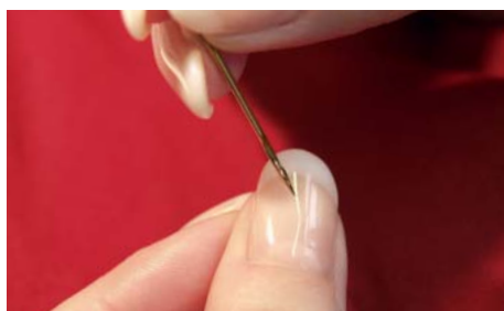
NEEDLE POINT TEST: DRAW NEEDLE POINT LIGHTLY OVER FINGERNAIL AND SEE IF IT LEAVES SCRATCH MARKS.
